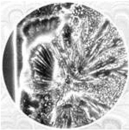
Microscopic View Untreated Hard Water (Mineral deposits after evaporation)
